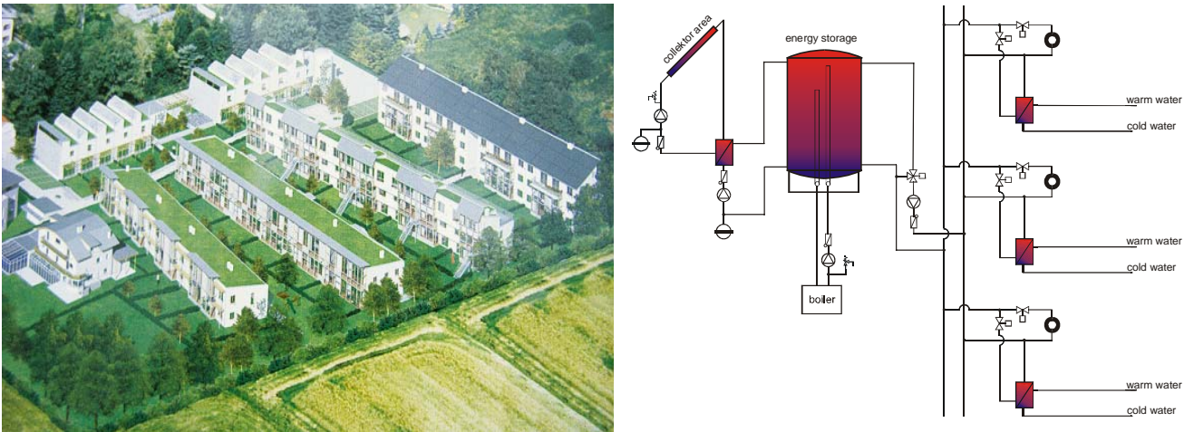
Fig. 8: General view of the housing estate Gneis-Moos (left) and the heat distribution system: Two-pipe-network with decentralised heat stations in each apartment (right).
